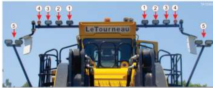
Front light locations (cab light bar lights) (Mounted each side of cab) (light type may vary)
