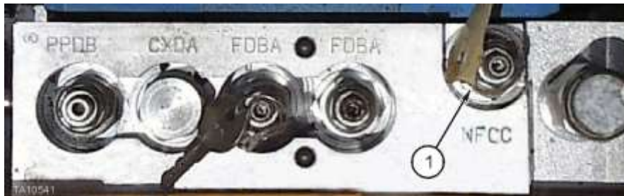
Manual release (Located on ladder control panel at top of ladder)
