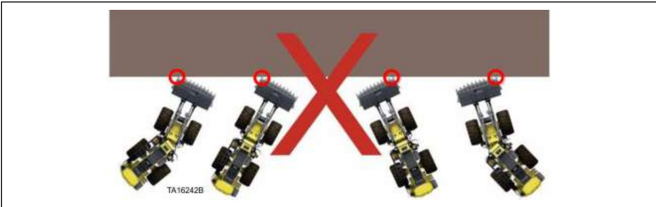
Figure 60. Do not corner dig
