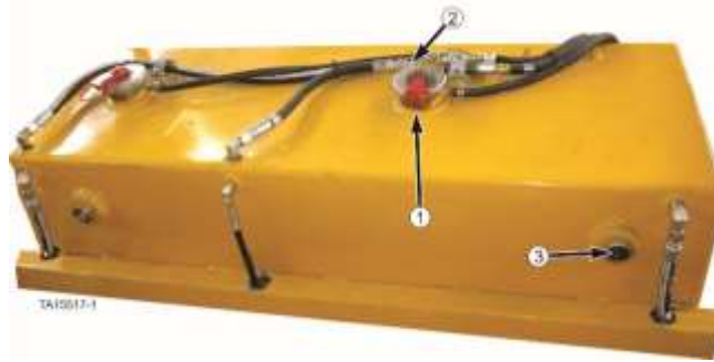
1) Radiator Cap, 2) Manual Pressure Relief Valve, 3) Sight Glass
