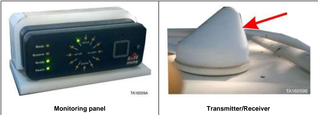
Figure 16. Typical proximity detection system components
