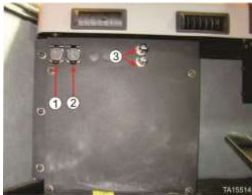
1) Ethernet Connection, 2) USB Connection, 3) Power-Ports
