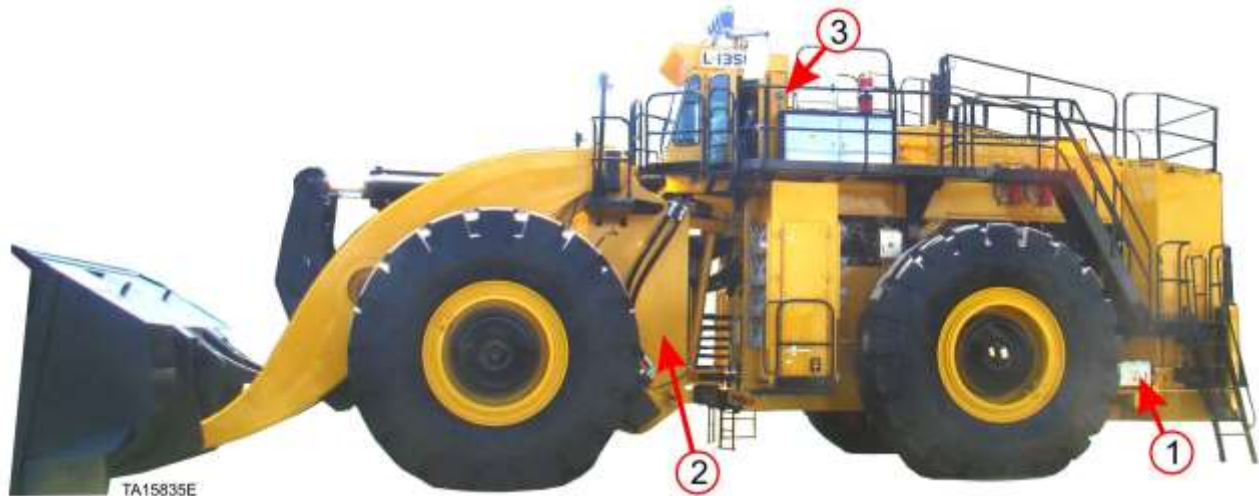
Figure 35. Battery isolator indication light and battery isolation switch
